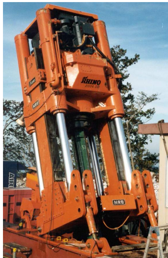
Fig. 2: The specially commissioned Rhino raise boring machine
