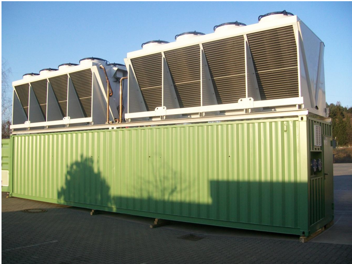
Freeze plant with condensers shown assembled and ready for shipment
